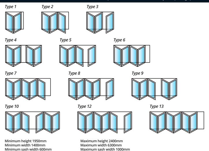
All configuration have lever/lever handles on the prime leaf with the exception of types 1, 4, 6 and 13 which are internal handles only.
